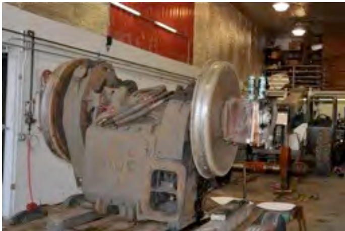
#1 axle combo preparing to separate the wheel/axle from the traction motor. Below: Bearing caps removed revealing the brass axle support bearings. These are the old style with a large window opening with the axle visible in the "window". Below right: New wheel (rusty one) being prepped for installation and old wheel in background.
