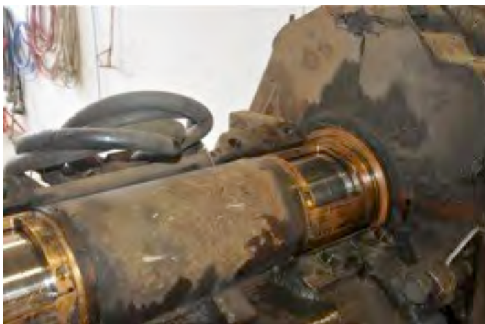
#1 axle combo preparing to separate the wheel/axle from the traction motor. Below: Bearing caps removed revealing the brass axle support bearings. These are the old style with a large window opening with the axle visible in the "window". Below right: New wheel (rusty one) being prepped for installation and old wheel in background.
